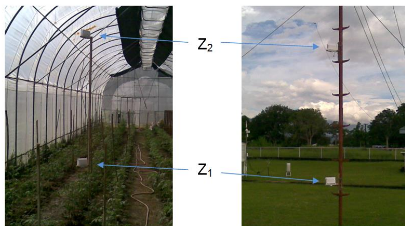
Figure 3-4. Data logger set-up for Bowen ratio measurement.
